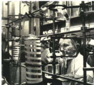
TAGGING PRODUCTS of tobacco smoke with radioactive carbon, scientists at the Medical College of Virginia hope to find out what parts of the body each component affects and in what way they are affected.
