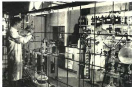
SPLITTING TAR into fractions in search for cancer-causing agent is done at New York University, partly supported by the Bureau of Food. Tar is first dissolved in big flasks (left), then heated. Finally the ingredients can be drawn off separately.
