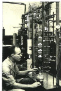
ISOLATING INGREDIENTS of cigaret smoke, a chemist at American Tobacco Co. lab collects each in vertical series of flasks.
