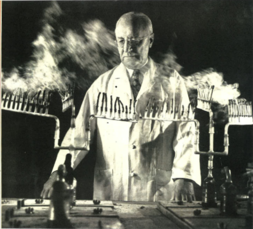
SMOKING MACHINE puffs on 60 cigarettes in front of Dr. Erastus Graham, who, with his collaborate on the mouse cancer research, Dr. Ernest Wynder, perfected the robot. The arratorator simulates the smoking inuater of humans
