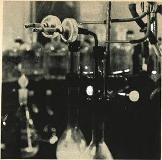
CU's tests of cigarettes over past years have been made with the apparatus shown above. What CU has learned has been that brands vary widely and change frequently with respect to tars and nicotine in the smoke taken in by the smoker. It is probably some of the tars which do the damage so far as lung cancer is concerned. But in this area of precisely how the smoking-lung cancer link is forged, more is to be learned than is known
