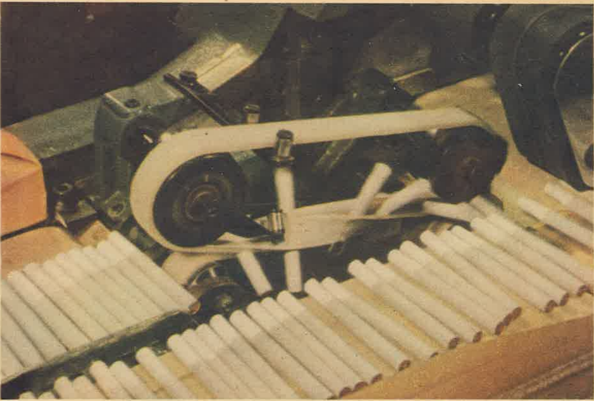
FILTER CIGARETTES —in this case KENTS—come from the making machine joined at the tip, two by two. Cut apart, half of them are turned over by this automatic belt so that all can be packed pointing the same way: filter end up.
