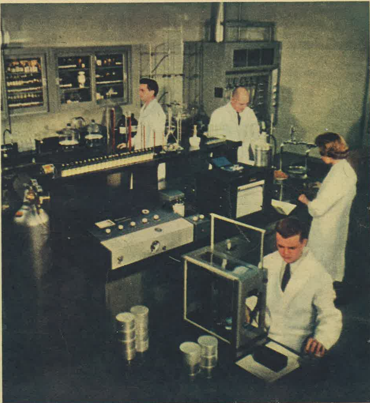
VARIETY of Lorillard equipment in a corner of one Greensboro laboratory includes analytical balance (right foreground) and (counter-clockwise) gas chromatograph, torsion balance, laboratory hood, distillation apparatus for solvent purification.
