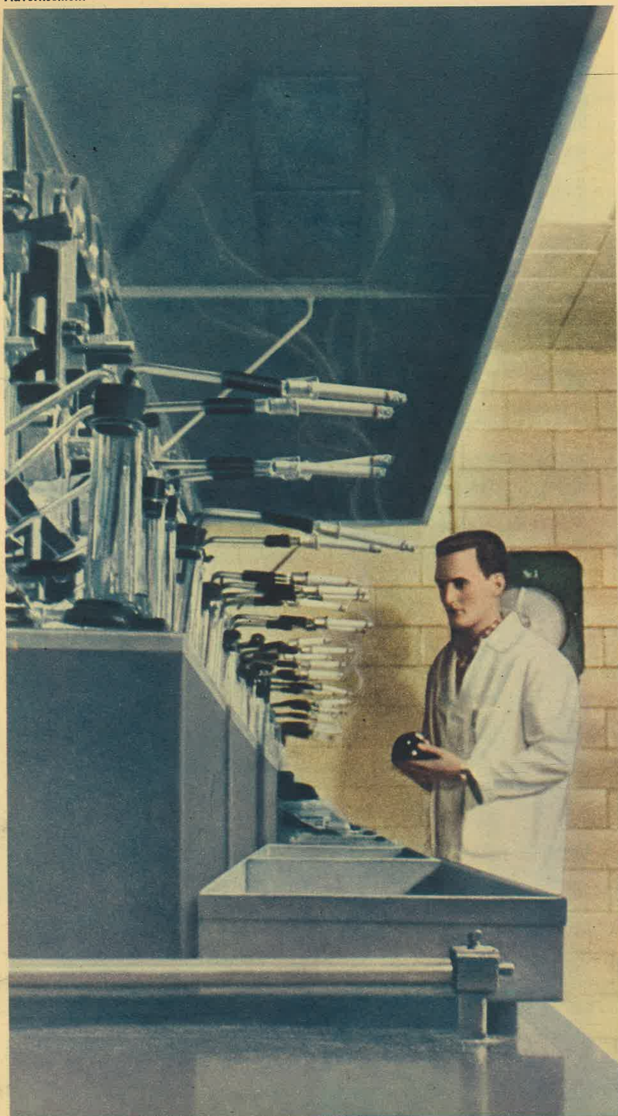
THREE DOZEN AT ONCE: Lorillard-designed "smoking machine" takes one puff a minute—the average smoker's rate—from each of 36 cigarettes. Flasks collect small amounts of condensate—the "raw material" for basic research on cigarette smoke.
