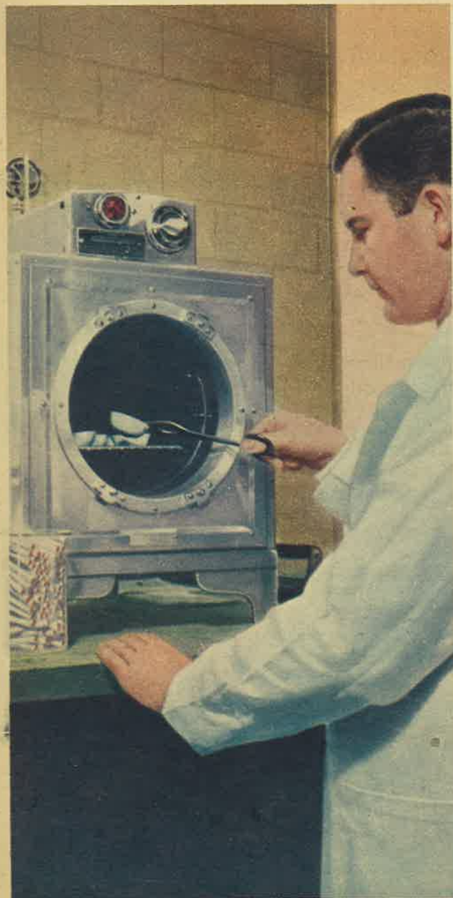
ELECTRIC FURNACE is used to reduce nicotine salt, isolated from tobacco, to ash. Weighed, ash indicates nicotine content.
