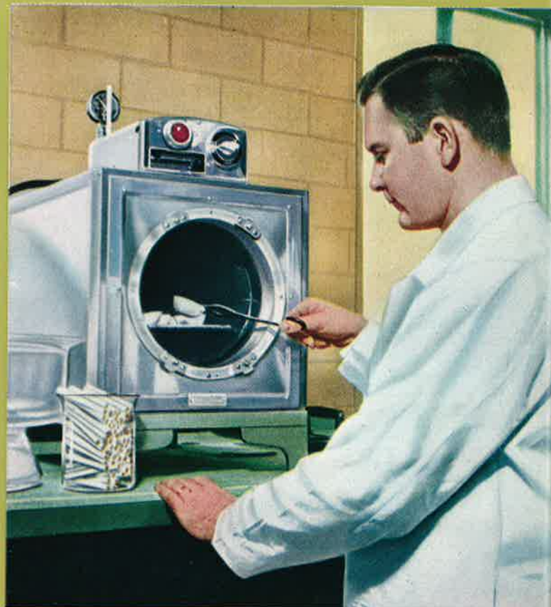
Miniature electric furnace is essential part of research apparatus. Here, nicotine salt is isolated, reduced to ash.
