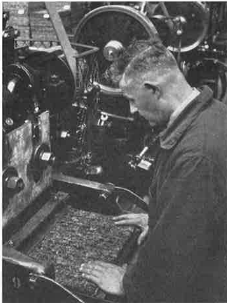
Flake tobacco going under the cutter
