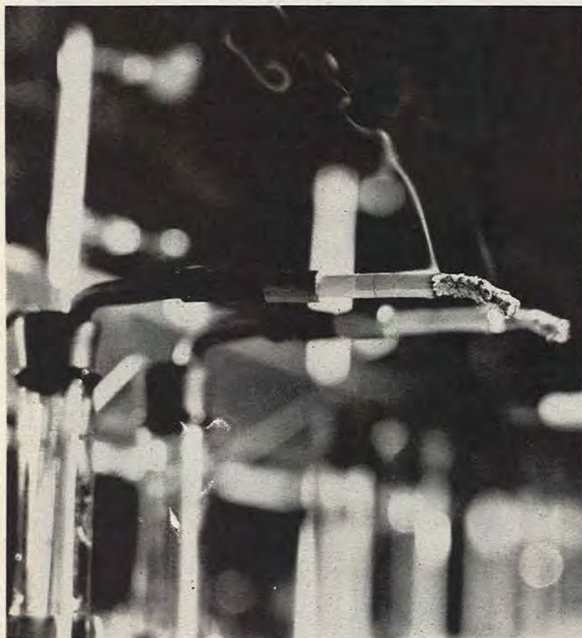
At P. Lorillard Co. lab cigarettes are smoked by machines which collect smoke and condense it to solid form so chemists can analyze contents.
