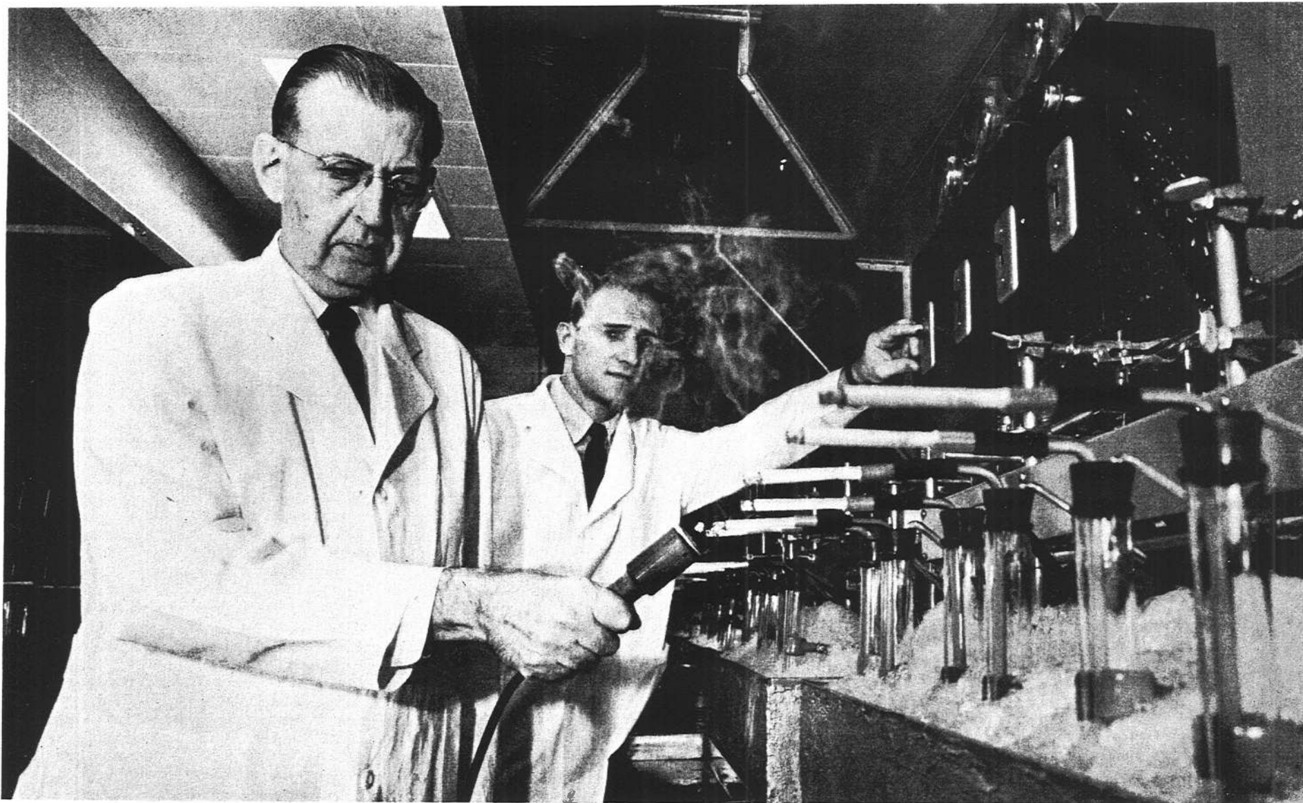
At P. Lorillard research laboratory in Greensboro, N.C., Drs. Clifford O. Jensen and Alex Spear light up a line of cigarettes in test smoking machine.
